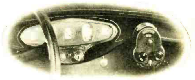
Fig. A The position of the Bosch radio control unit is shown at the right of a standard auto instrument panel. The knobs are tuning and volume controls.
